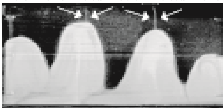
Fig. 15. Convection driven by two layers of miscible fluids submitted to a temperature gradient. For intermediate values of the stabilizing chemical density anomaly to the destabilizing thermal density anomaly, large domes develop and oscillate vertically through the whole layer. Thin plumes rise from the upper surfaces of the domes (white arrows) (Davaille, 1999).
