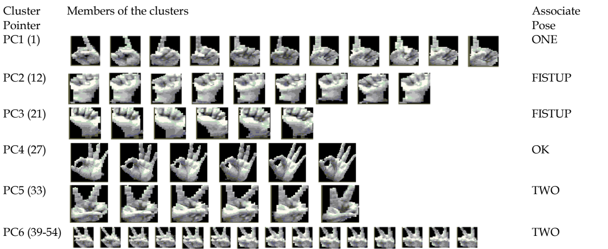
Fig. 12. Example output of multi-clustering approach for learning new pose
