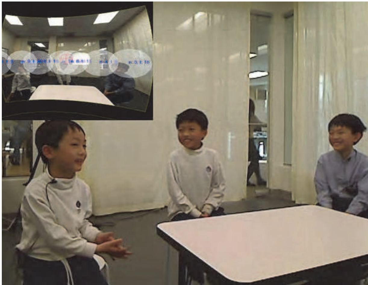
Fig. 8. Automatic logging of speaker activity and locations for multi-speaker applications: (inset) Panoramic attention locates speakers and logs amount of speaker activity for each participant. White circle regions represent past clusters of sound activity labeled with current number of utterances and cumulative time spoken.
