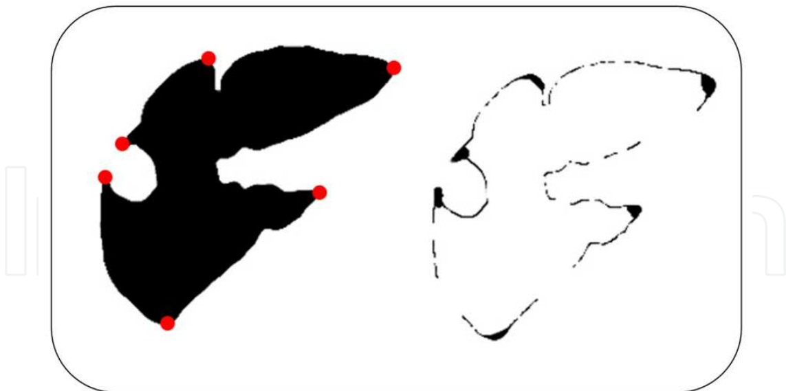
Fig. 12. Identifying the outstanding corners around liver structure
