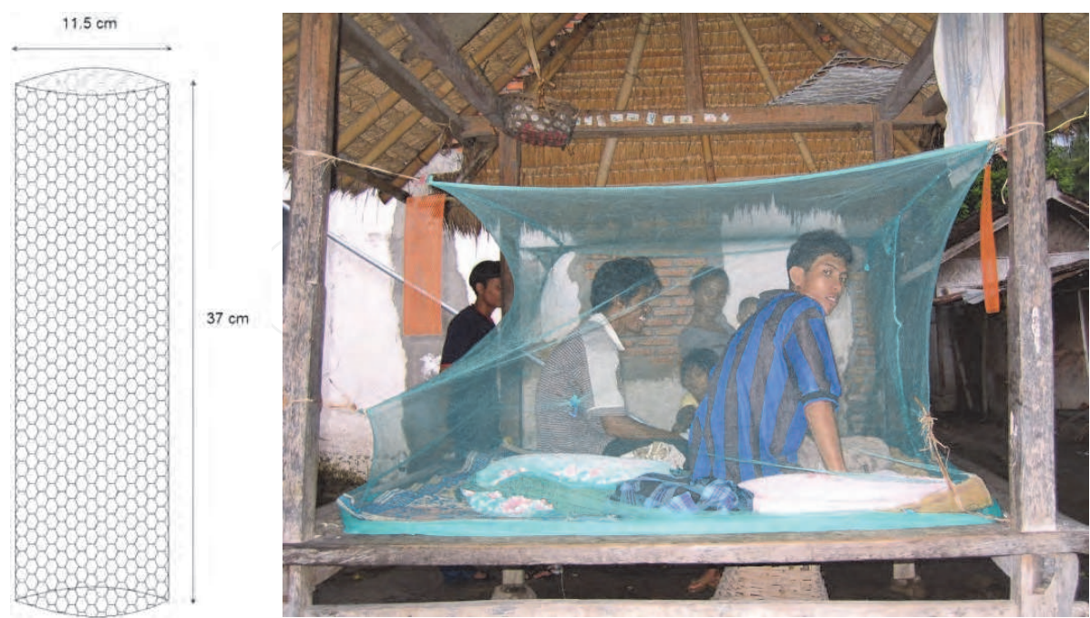
Fig. 3. Metofluthrin-impregnated plastic strip for the trial and the field test scene with the strips in a beruga where Lombok people spend every evening before going to bed (Kawada et al., 2005a).
