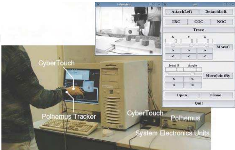
Fig. 10. An example of the client setup, and a snapshot of the GUI with a window displaying sensory information received from the remote site.
