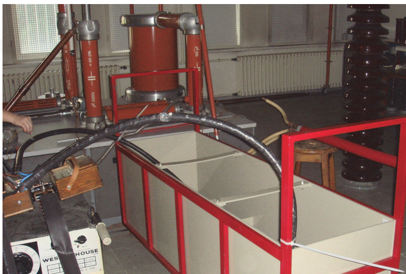
Fig. 15. Experimental set-up for 0.6/1 kV cable.
