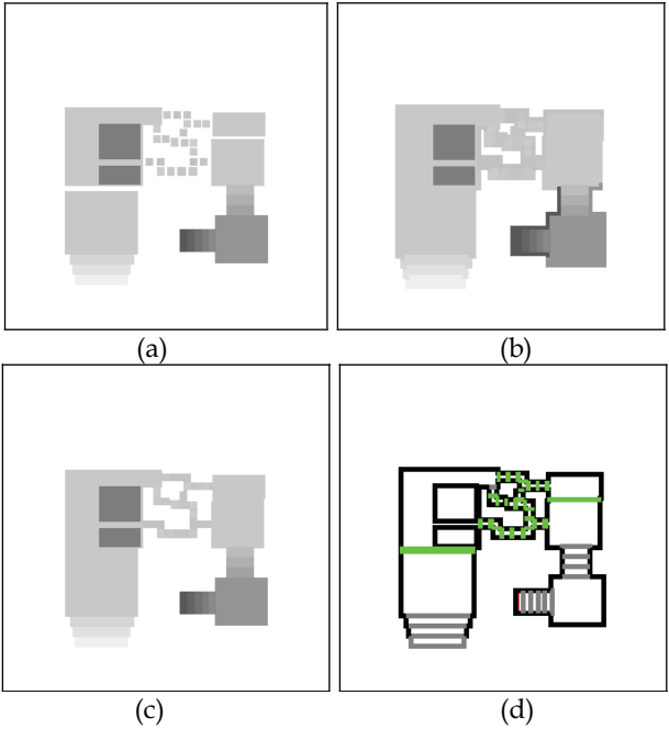
Fig.5. (a) height map for the environment in Fig. 1., (b) map in (a) after applying dilation, (c) map in (b) after applying erosion. After the closing operator, the columns in the discontinuous region are connected. (d) instability map
