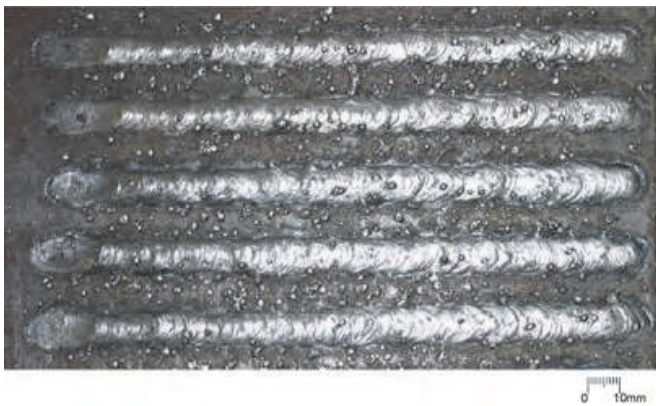
Fig. 10. Beads on plate performed by the robot using E6013 electrodes, demonstrating the repeatability of the process.
