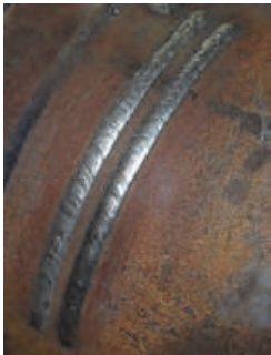
Fig. 13. Welds made on tube with E7018 electrodes.
