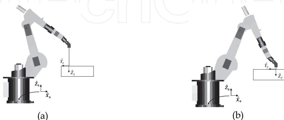
Fig. 4. Initial (a) and final (b) robot positions during shielded metal arc welding for a 90^\circ welding angle.
