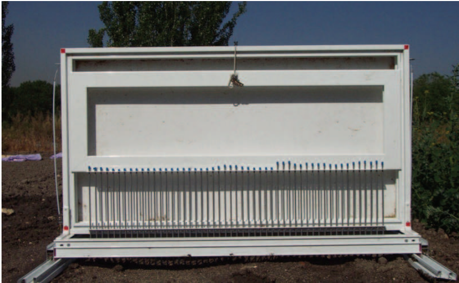
Fig. 1. Pin-meter used to measure soil surface roughness
