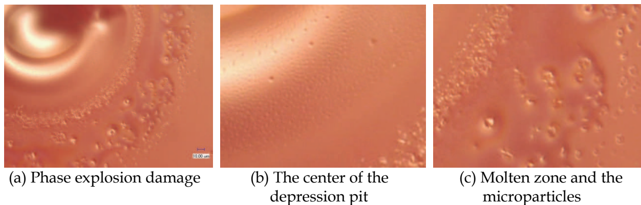
Fig. 2.8. Damage morphology induced by phase explosion (15kHz)
