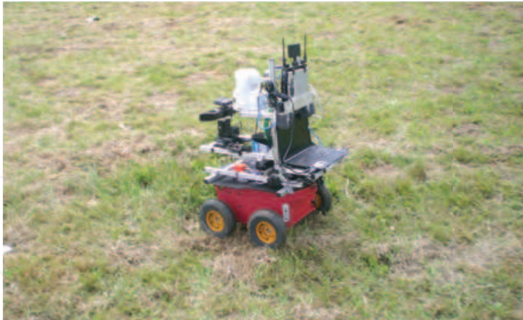
Fig. 8. Robot PIONEER 3AT equipped with Kinect sensor. Photo taken during Land Robot Trial CELROB 2011.
