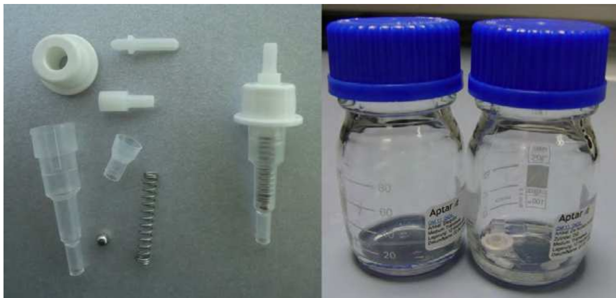
Picture 1. Parts for a standard pump and how it looks like when assembled. On the right side: soaking of parts in formulation to check compatibility. For demonstration just parts for one pump are depicted.
