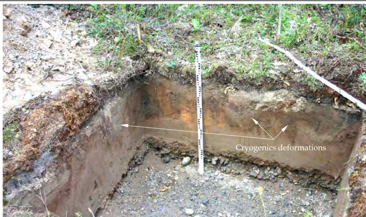
Fig. 19. Cryogenics deformations in floodplain deposits of the Angara-Tunguska off-glacial zone (Northwestern glaciations unit; left bank of the Kirenga River in the vicinity of the settlement of Magistralny, pit No. 5).
