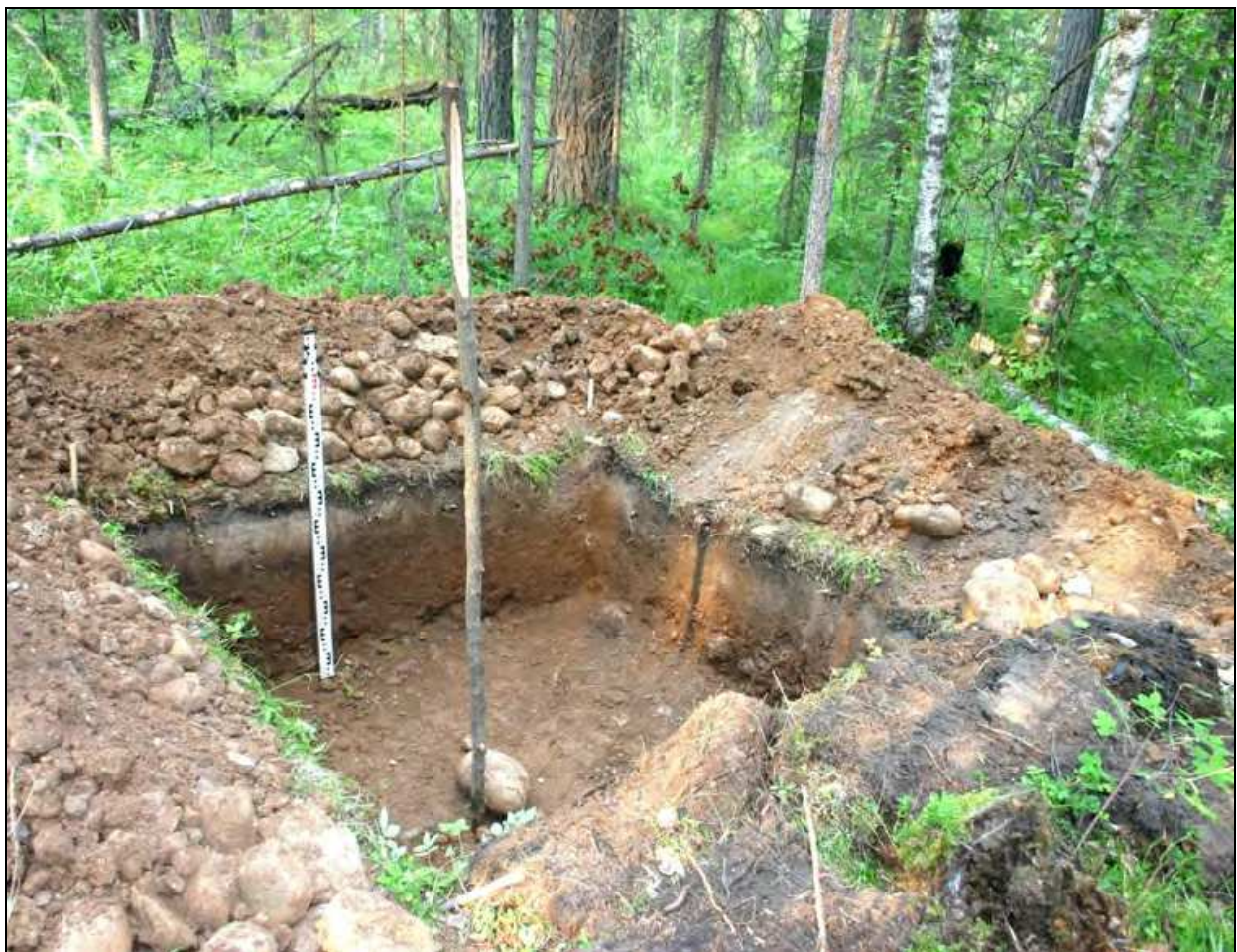
Fig. 10. Morainic boulder-block-pebble deposits in clayey cement. Northwestern glaciations unit; pit No. 64 is located in the mouth zone of the Minya River (the right tributary of the Kirenga River).
