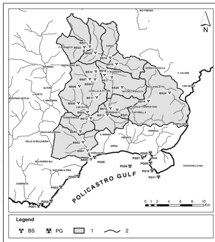
Fig. 4. The Bussento river basin monitoring network. BS is the symbol for streamflow stations whereas PG is the symbol for marine stations, for discharge and radon measurements.
