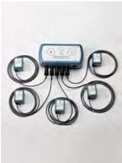
Fig. 2. Kinetisense, Cleveland Medical Devices Inc. system for PD monitoring based on motor sensors and electromyography (Jovanov et al., 2001)
