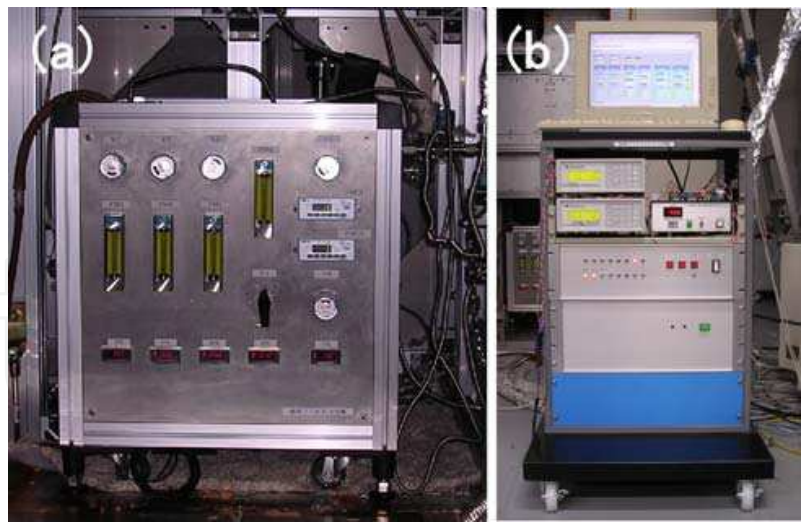
Fig. 12. Hardware of the gas control system of the HCS (a), and computer to control the gas flow together with temperature minitors and Liquid helium level meter (b).
