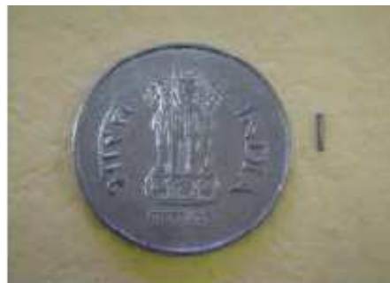
Fig. 7. Encapsulated ^{125}\text{I} - brachytherapy sources
