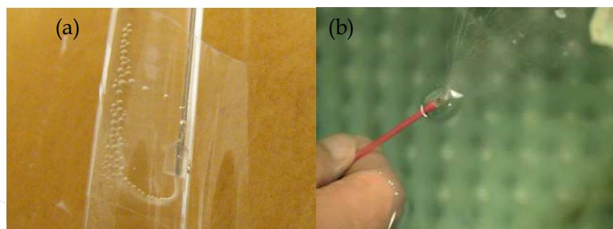
Fig. 12. Acoustic cavitation (a) and acoustic streaming (b)
