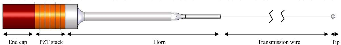
Fig. 9. Schematic illustration of the piezoelectric thrombolysis device
