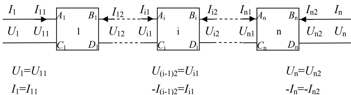
Fig. 4. Finite electrical circuit element model
