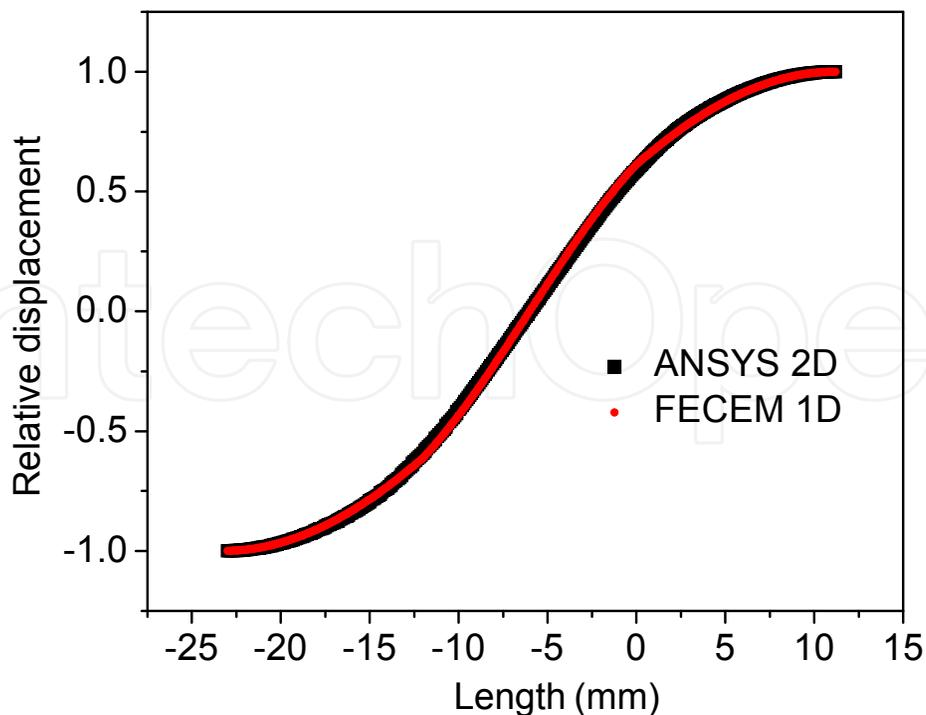
Fig. 5. Comparison of mode shape of Langevin transducer
