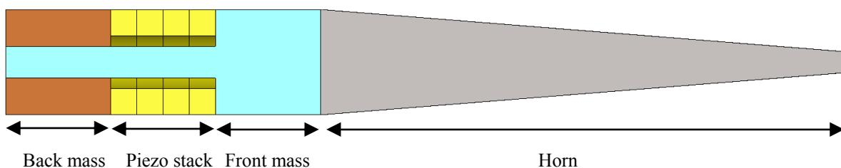
Fig. 1. General structure of a horn-type piezoelectric transducer
