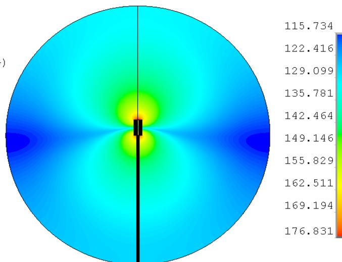
Fig. 11. Acoustic pressure pattern generated by the tip in the liquid
