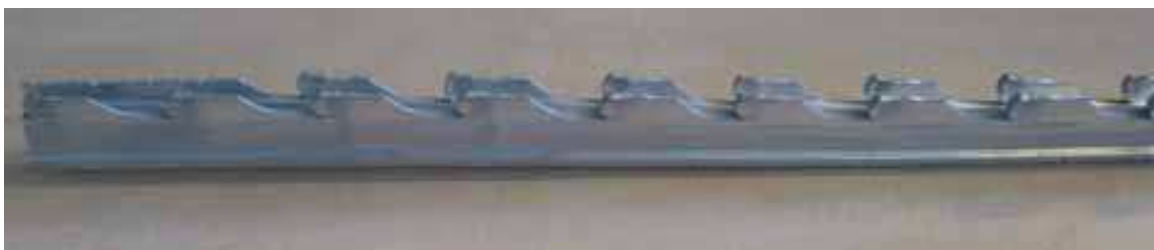
Fig. 1. Extreme case of hot tearing in AA7075 aluminum alloy [3]
