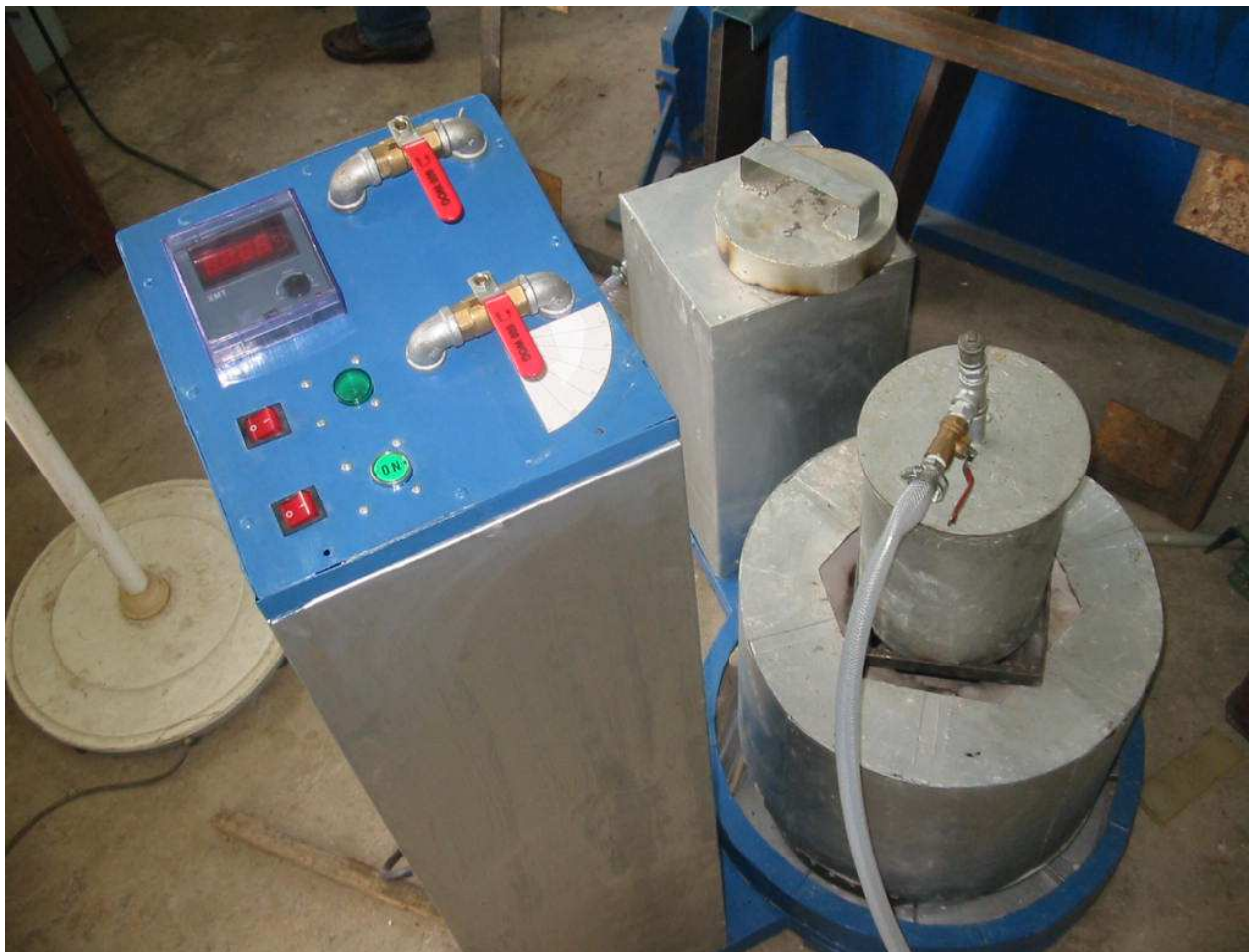
Fig. 13. A low-cost machine for countergravity casting
