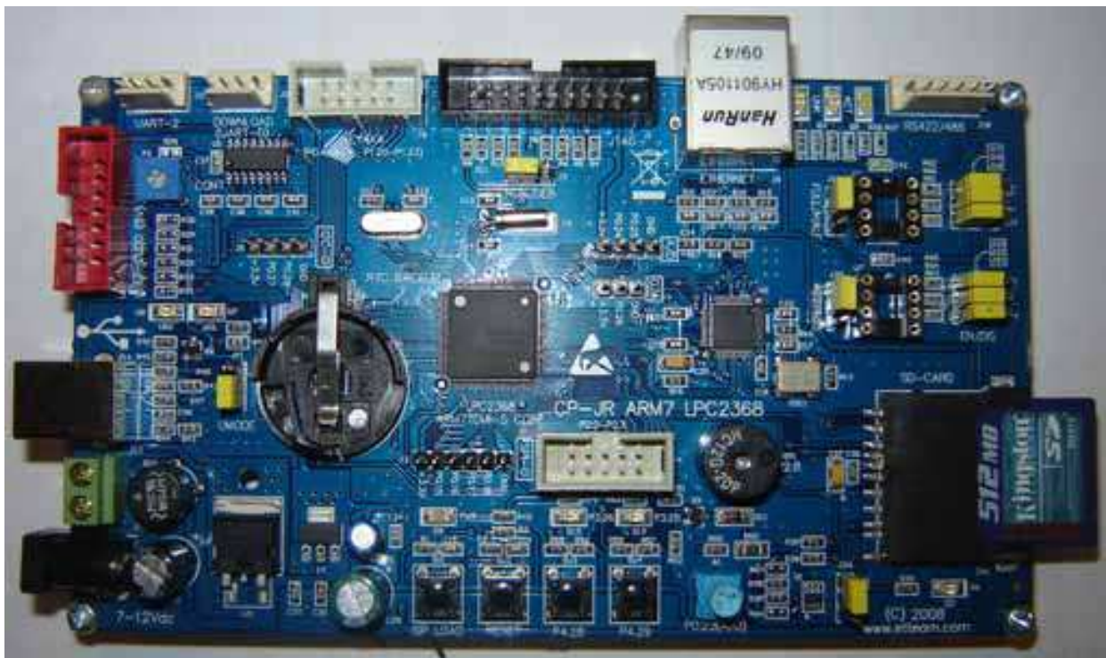
Fig. 5. The development board of LPC2368 microcontroller
