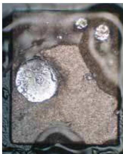
Fig. 18. Solder joint structure, cross-section view
