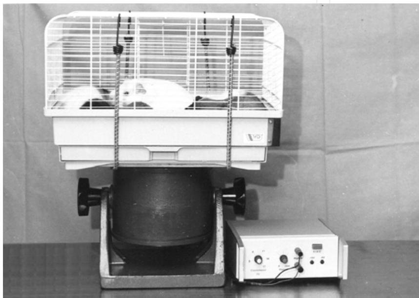
Fig. 9. Cage with animals exposed to vibrations
