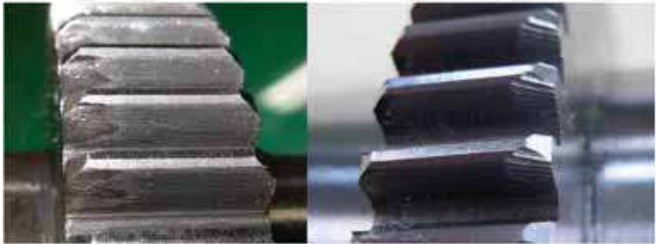
Fig. 8. Gear tooth worn by misalignment
