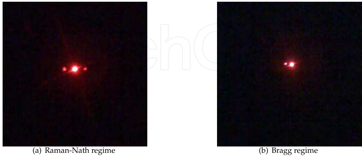
Fig. 17. Output beam diffracted by the AOD under different interaction regimes
