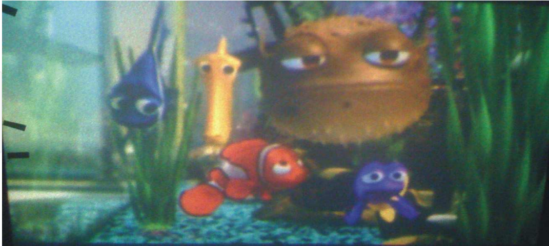
Fig. 8. Projected image at WVGA resolution resulting from a phase-only holographic projection system, employing the techniques described in this chapter, manufactured by Light Blue Optics Ltd. In this instance, \lambda_r = 642 \text{ nm} , \lambda_g = 532 \text{ nm} and \lambda_b = 445 \text{ nm} .
