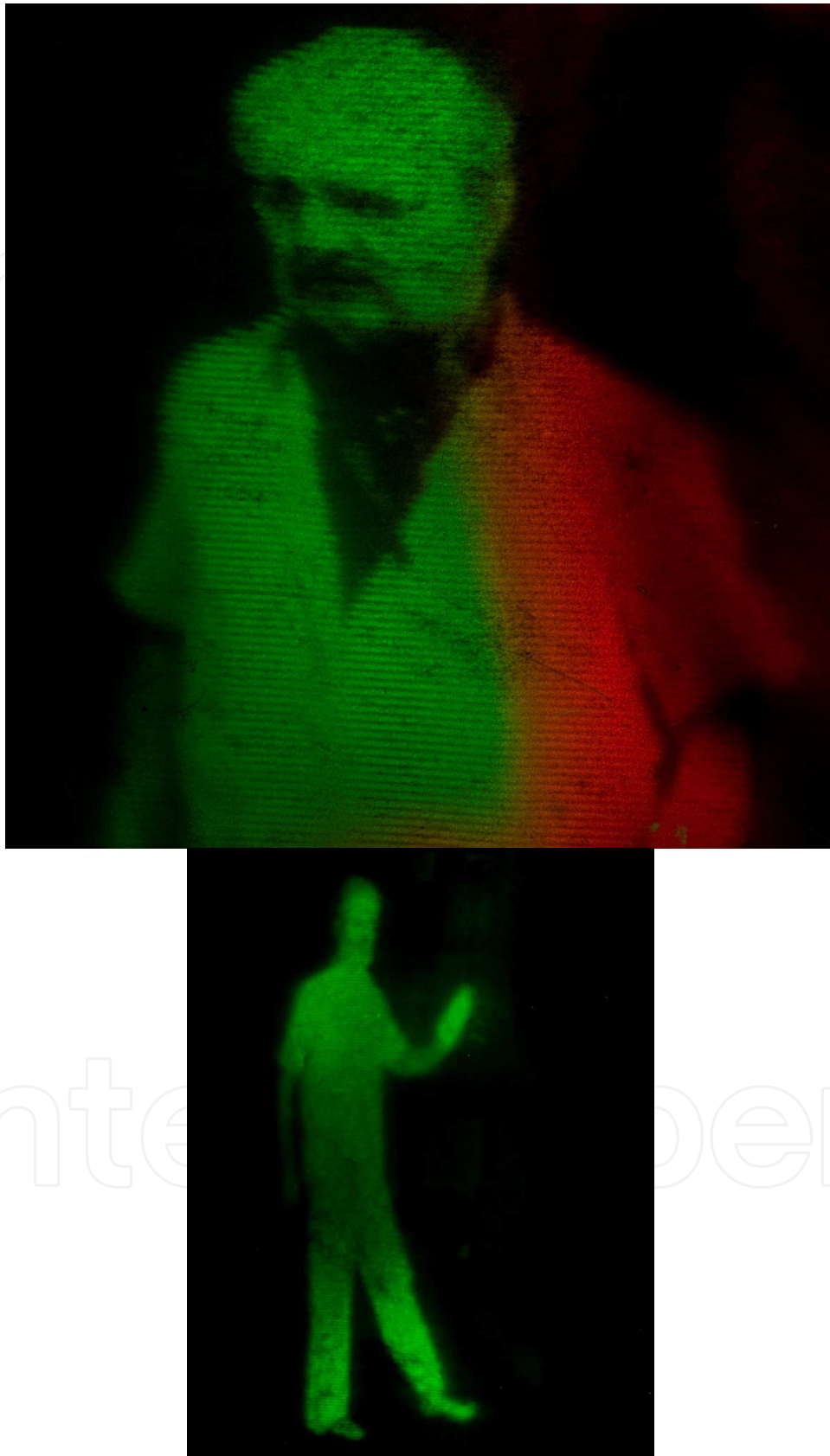
Fig. 8. Vídeo scene appearing in an oblique plane in front of the screen. a) detail. b) complete image, 80 cm high, made of two hundred video lines.
