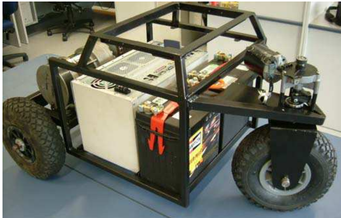
Figure 9. Complete chassis and drive components
