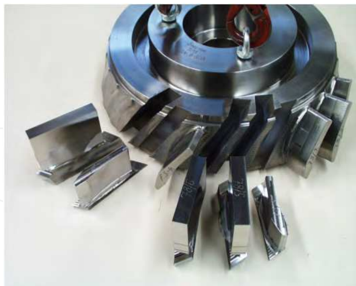
Fig. 26. Pre-machined BLISK demonstrator, after extraction of blade-blocks.
