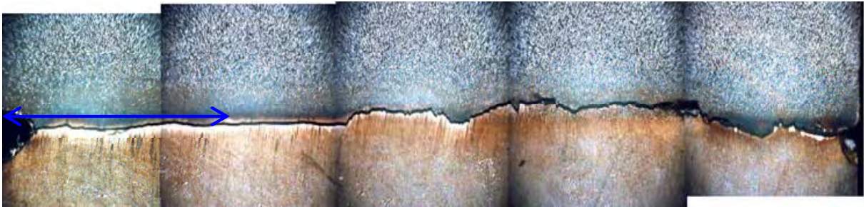
Fig. 23. Crack path for fracture toughness specimen corresponding to K_{Ic} = 15 \text{ MPa.m}^{1/2} .
