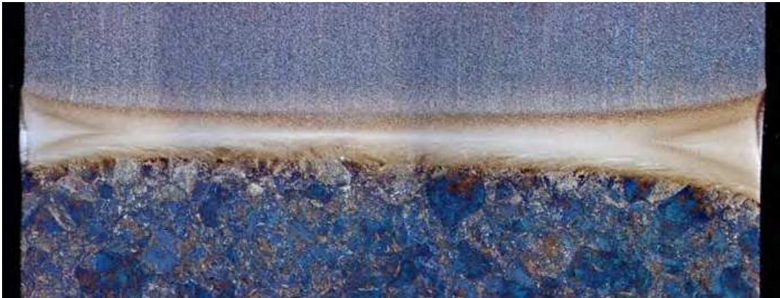
Fig. 12. Macrograph of the cross section of a weld (blade material in the upper part and disk material in the lower part).
