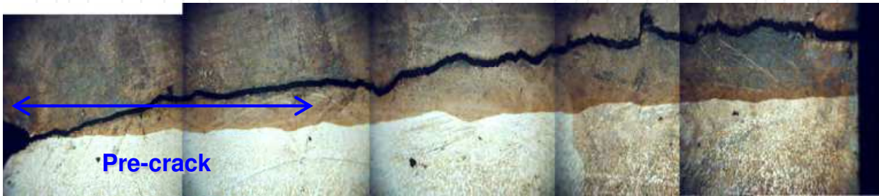
Fig. 24. Crack path for fracture toughness specimen corresponding to K_{Ic} = 45 \text{ MPa.m}^{1/2} .
