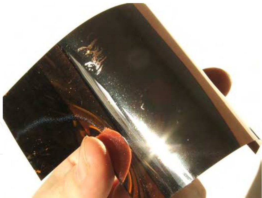
Fig. 14. Test structure of elastic CdTe layer based on UPILEX® foil and contacted by 2 \mu\text{m} Cu layer.
