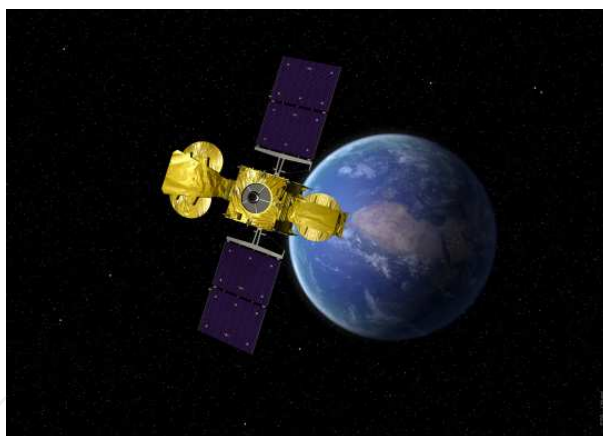
Fig. 19. Deployable Solar panels, Hylas-1 (Credits: ESA - J. Huart.)
