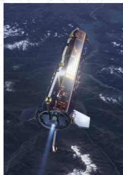
Fig. 18. Body mounted solar array, GOCE (Credits: ESA - AOES Medialab)
