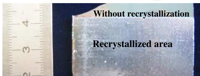
Fig. 3. Appearance of polycrystalline silicon absorber after recrystallization
