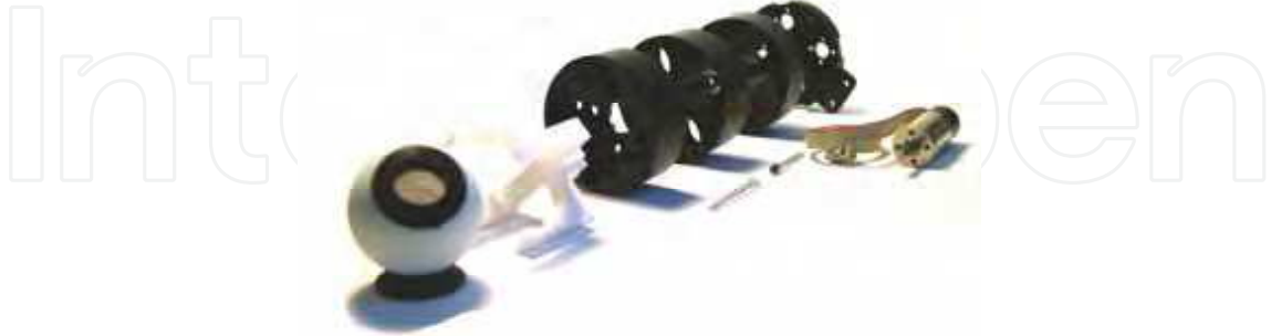
Fig. 16. The body of the MAC-EYE robot. All the motors are integrated within the body; furthermore, all the cables from and to the eye-ball and the embedded optical tension sensors are routed inside of the structure.
