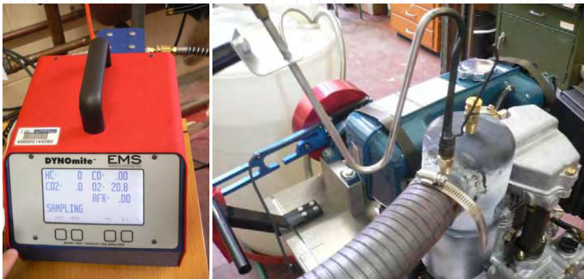
Fig. 9. Gas Analyser and emission probe
