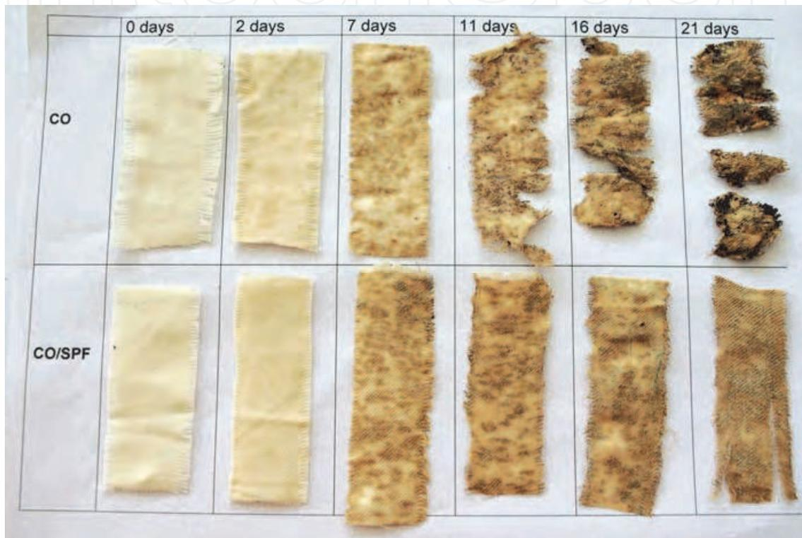
Fig. 11. Fabric samples after having been buried in the soil for 0 to 21 days. (Photo: Marica Starešinič)
