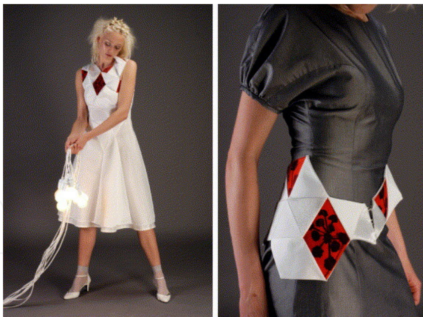
Fig. 10. An example of patterned polymer solar cells on a PET substrate incorporated into clothing by sewing through the polymer solar cell foil using an ordinary sewing machine. Connections between cells were made with copper wire that could also be sewn into the garment. The solar cells were incorporated into a dress and a belt. Design by Tine Hertz Reprinted from Sol. Energy Mater. Sol. Cells, 90, Krebs F.C.; Biancardo M.; Jensen B.W.; Spanggaard H. & Alstrup J., Strategies for incorporation of polymer photovoltaics into garments and textiles, 1058-1067, Copyright (2006), with permission from Elsevier.
