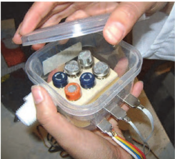
Fig. 3. The chamber of sensors provides hermetic isolation and guarantees reliable measurements.
