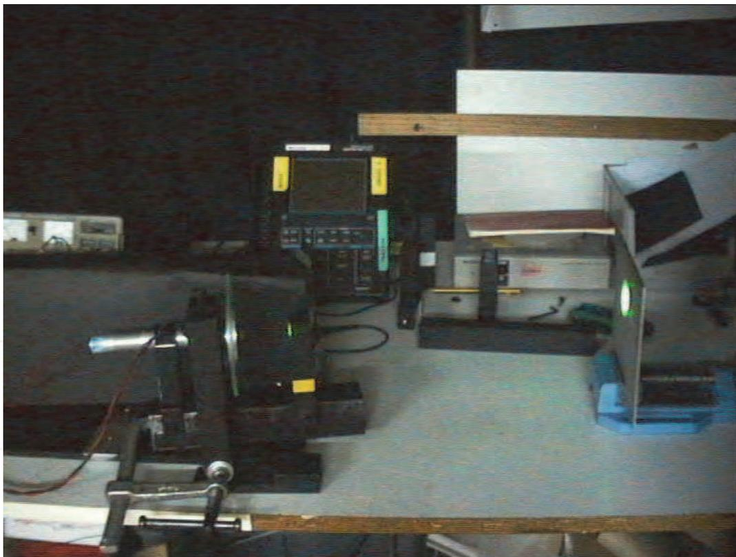
Fig. 3. Laboratory benchmark: diffuse bright-field lighting with a 160 mm focal length lens and a green DPSS laser.
