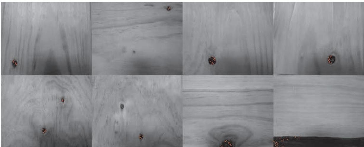
Fig. 6. Results of wood defect detection in images (first set) acquired with standard lighting visual system.
