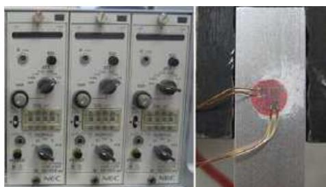
Fig. 14. Strain Gage and Amplifier
