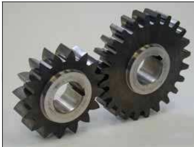
Fig. 12. Coated test gears used for testing scuffing - type A
