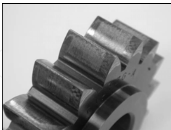
Fig. 1. A typical scuffing wear of gear teeth
