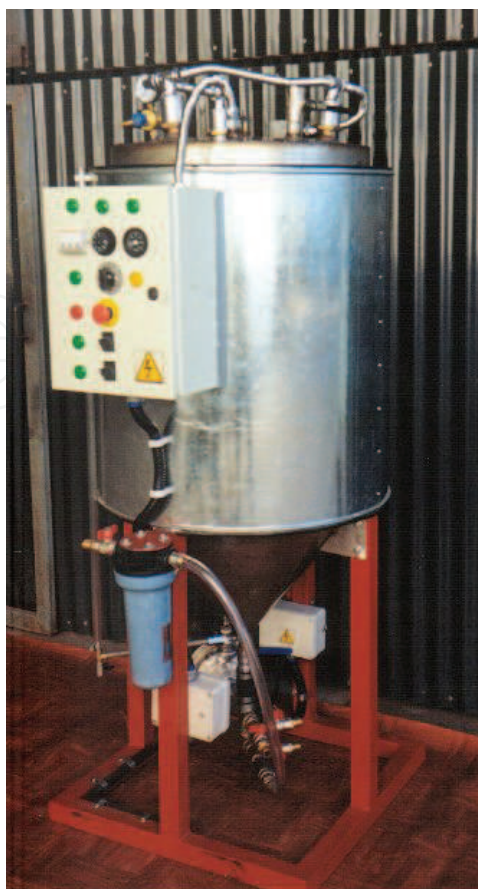
Fig. 8. Transesterification batch reactor
