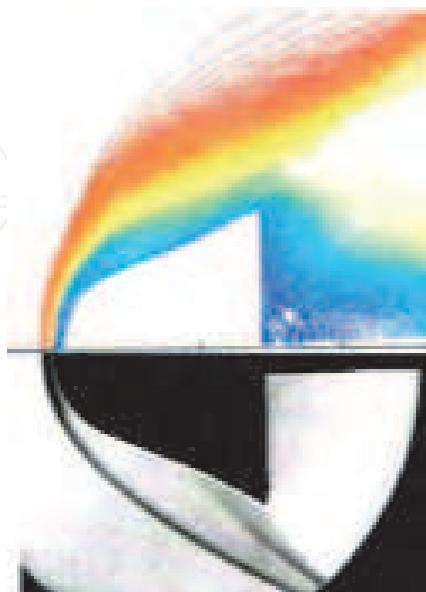
Fig. 4. Comparison between density contour and schlieren picture.
