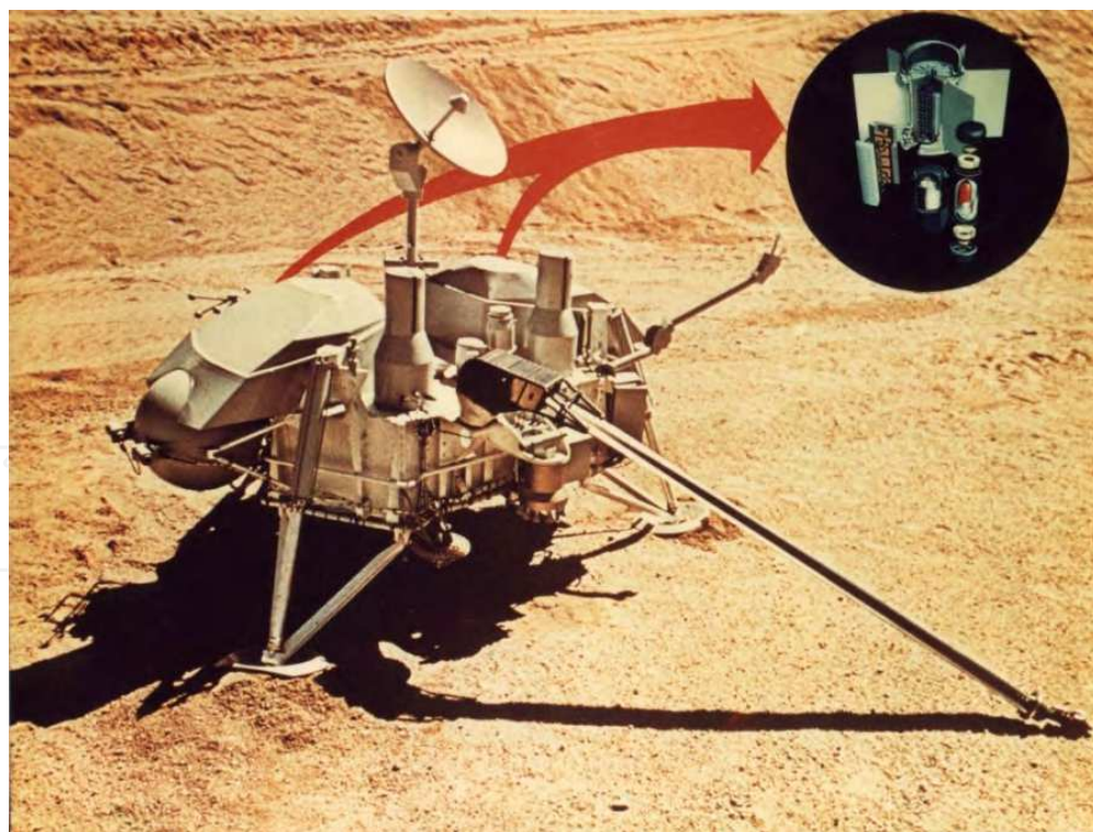
Fig. 6. Viking Lander model showing the location of the two SNAP-19 RTGs. The average power per RTG was 42.7 We at BOM. The overall RTG diameter (across fins) was 58.7 cm and the overall length was 40.4 cm. The mass was 15.2 kg. (Image credit: NASA/JPL/Caltech/ERDA/Teledyne)
