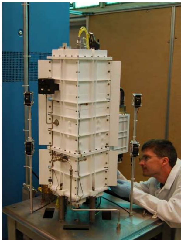
Fig. 18. ASRG engineering unit readied for extended testing at NASA Glenn Research Center (Photo Credit, NASA Glenn).
