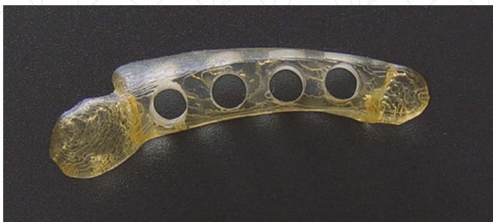
Fig. 6. Fabrication of the guide by stereolithography machine.
