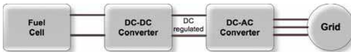
Fig. 19. A typical FC configuration with a DC-DC and a DC-AC converter
