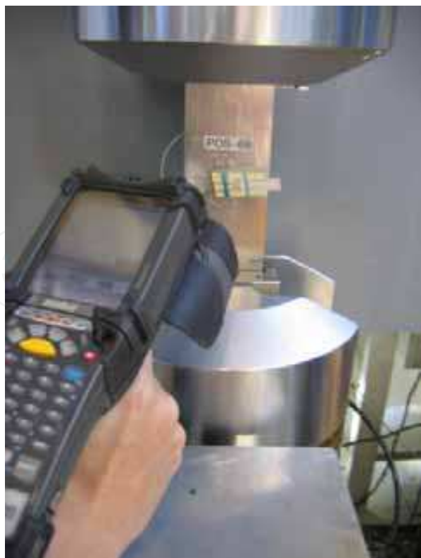
Fig. 20. Illustration of an RFID-based crack detection approach.
