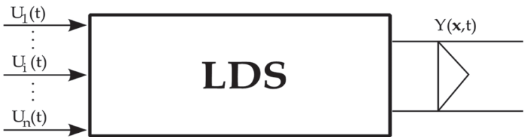
Fig. 2. Lumped-input and distributed-parameter-output system - LDS
