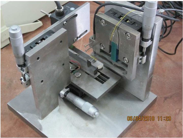
Fig. 21. Prototype of designed indentation device
