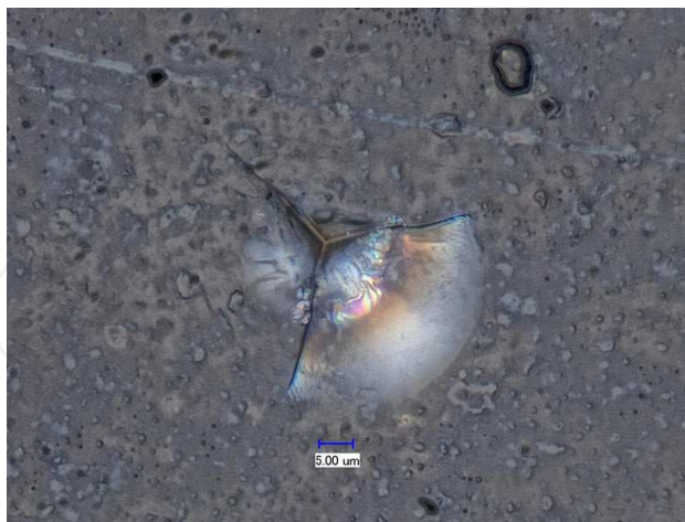
Fig. 37. Indentation morphology of optical glass
