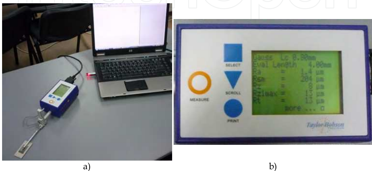
Fig. 32. The parameters calculated by “Surtronic 25”
