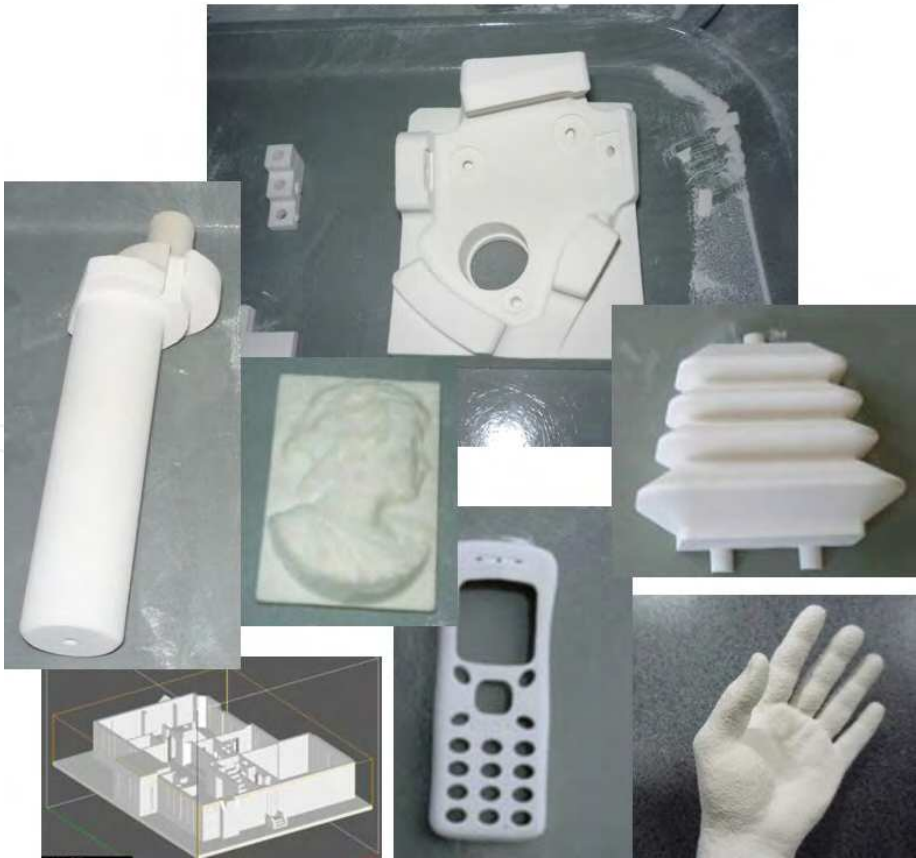
Fig. 28. Products obtained by “inkjet” printing (Z310 Plus), Transilvania University of Brasov
