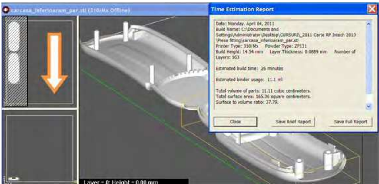
Fig. 22. Positioning of parts along Y axis, “XY-90°” rule satisfied (inkjet technology)
